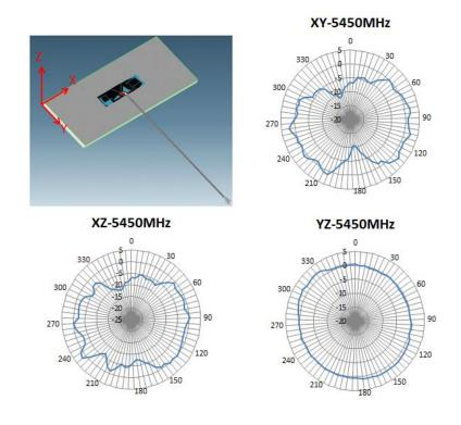
FIGURE 5.2 RADIATION PATTERN OF ANTENNA AT 5.45GHZ IN FREE SPACE
