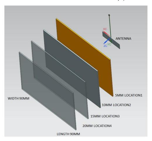
FIGURE 4.2 FOUR LOCATIONS WITH PARALLEL GROUND
