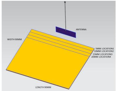
FIGURE 4.1 FOUR LOCATIONS WITH VERTICAL GROUND
