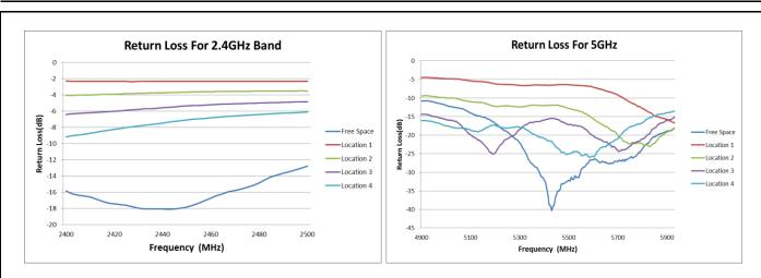
FIGURE 4.2.1 RETURN LOSS OF ANTENNA AT 2.4/5GHZ BAND AT FOUR LOCATIONS WITH PARALLEL GROUND
