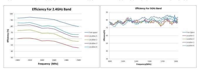
FIGURE 4.1.2 EFFICIATION OF ANTENNA AT 2.4/5GHZ BAND AT FOUR LOCATIONS WITH VERTICAL GROUND
