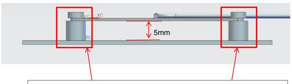
These two columnar materials can be plastic with metal nut or pure plastic. Pure metal is not recommended.
